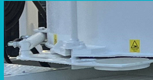
Hydraulic Gate Opening
